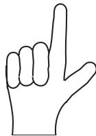
Start rope at right hand flange for right hand lay rope.
